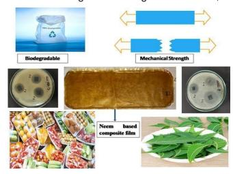
decrease in opacity value. Biodegradability studies were conducted by Soil burial method and the films demonstrated complete biodegradability within 75 days. The results of thermogravimetric analysis (TGA) and differential scanning calorimetry (DSC) of composite films show that they are thermally stable and might be used in food packaging.
